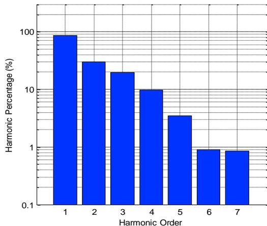
Figure 5. Harmonic in transformer currents
