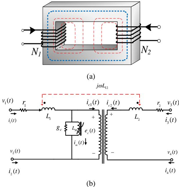
Figure 1. Single-phase transformer model: (a) two-winding transformer, (b) equivalent circuit.
