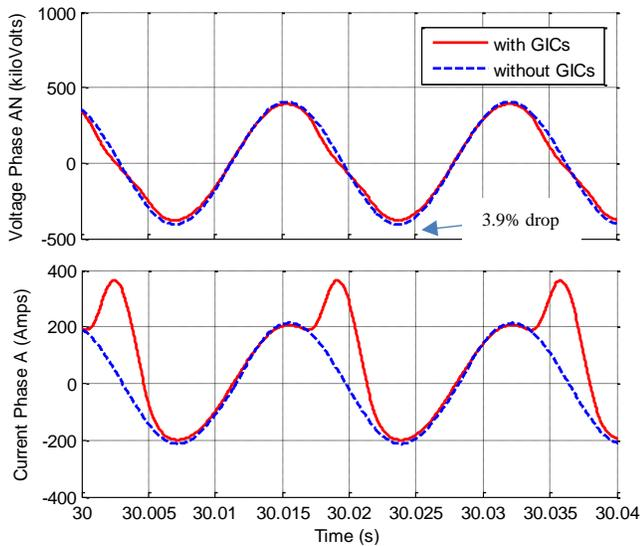
Figure 4. Impact of solar storms on transformer core saturation
