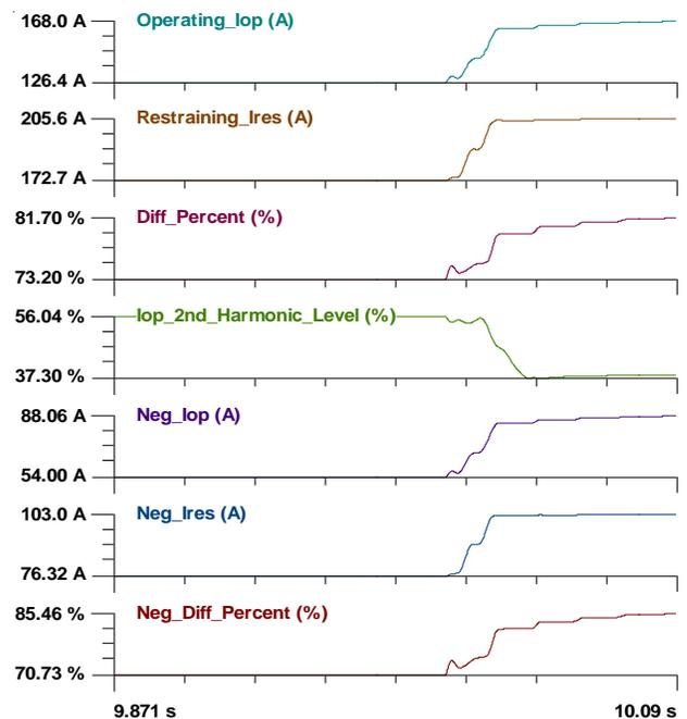
Figure 6. Percentage differential, harmonic-restraint differential and negative-sequence differential protection results
