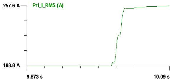
Figure 7. Result of overcurrent protection
