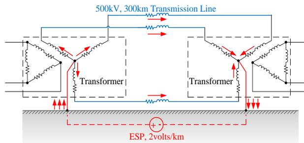
Figure 3. Test system for numerical simulations
