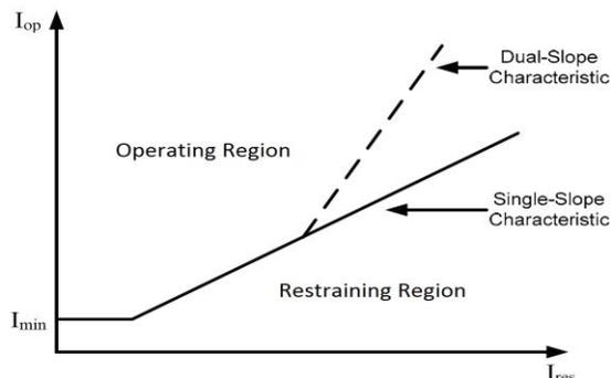
Figure 2. Percentage-differential protection method
