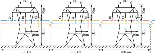
Figure 4. Tower structure of the Practically transposed line
