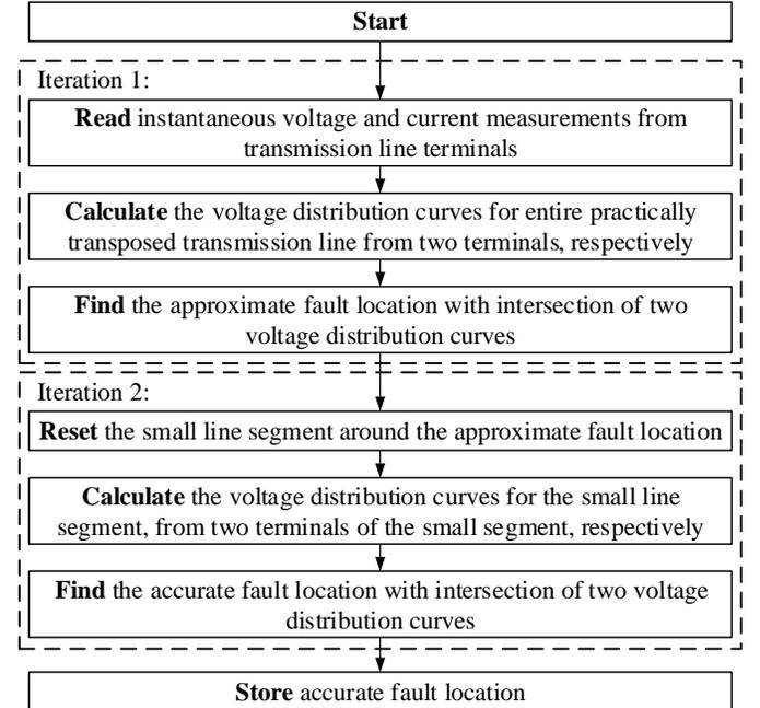
Figure 3. Flow chart of the fault location algorithm
