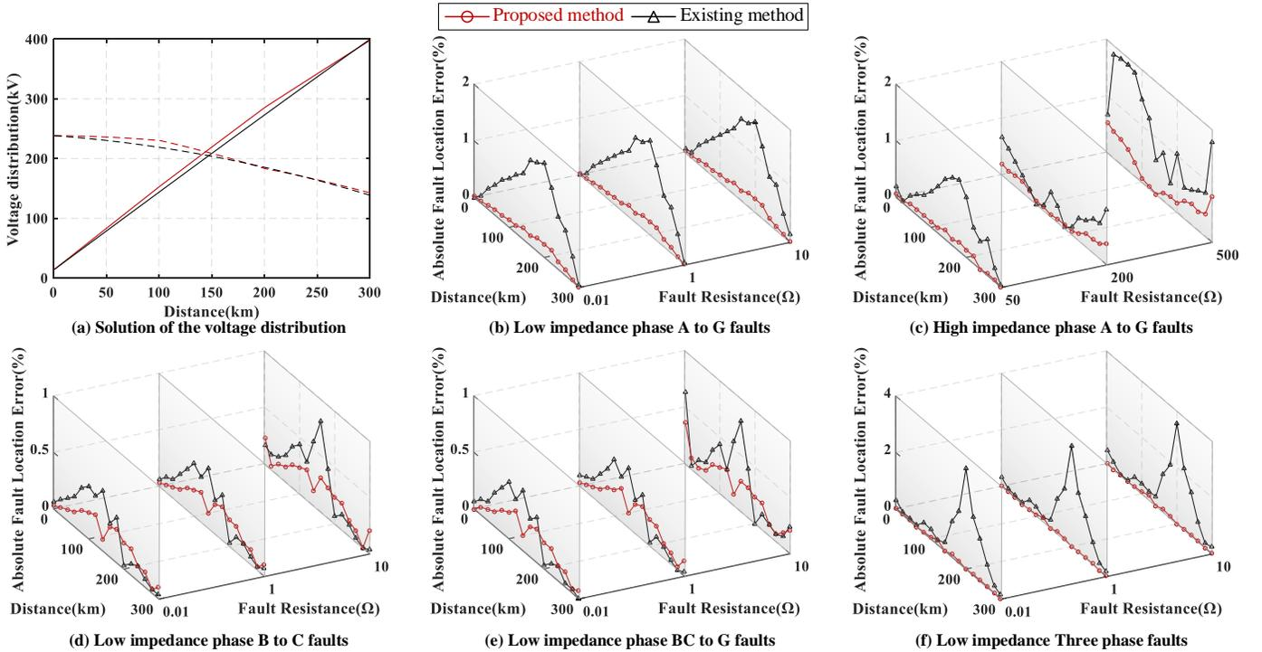
Figure 5. Solution of the voltage distribution and absolute fault location error with different fault types, fault locations and fault impedances
