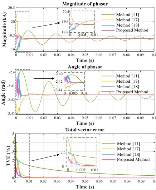
Figure 3. The magnitudes, phase angles and the TVEs of the estimated phasors, small dc offset
