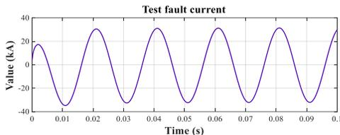
Figure 4. Fault current signal during SLG faults, large dc offset
