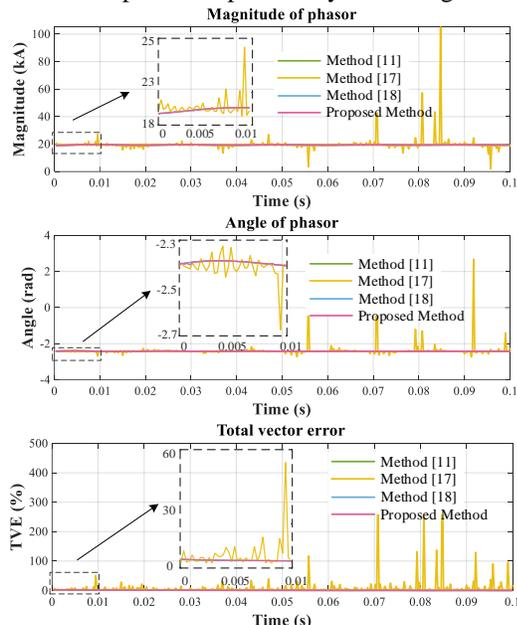
Figure 7. The magnitudes, phase angles and the TVEs of the estimated phasors, 2% measurement noises
