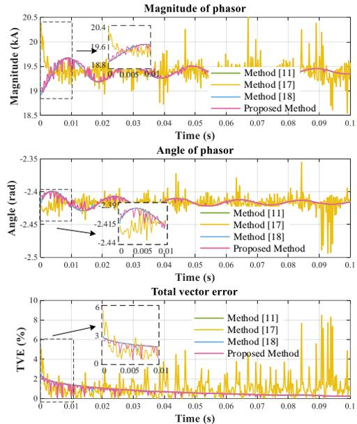
Figure 6. The magnitudes, phase angles and the TVEs of the estimated phasors, 0.5% measurement noises
