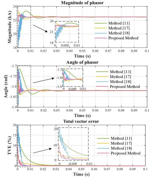
Figure 5. The magnitudes, phase angles and the TVEs of the estimated phasors, large dc offset
