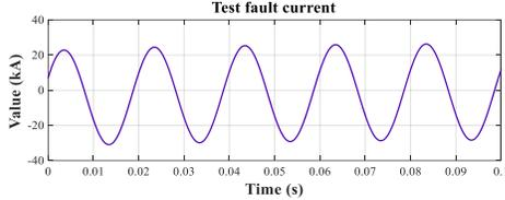
Figure 2. Fault current signal during SLG faults, small dc offset
