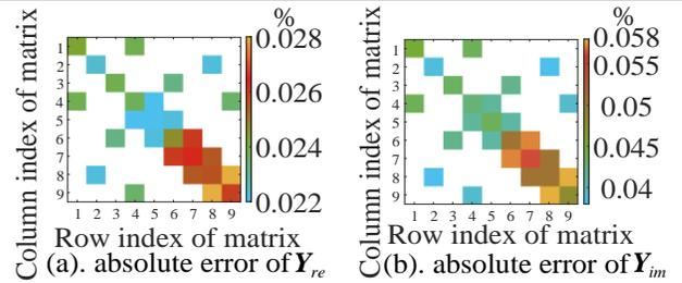
Figure 4. Absolute error of  $Y_{re}$  and  $Y_{im}$ , 9-bus system
