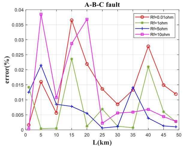
Figure 7. Results of the absolute fault location errors (in percentage), low impedance phase ABC faults with different fault locations and fault impedances
