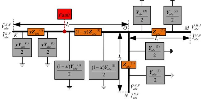
Figure 2. The three-terminal line model during the fault
