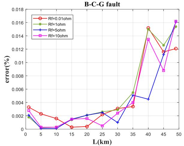
Figure 6. Results of the absolute fault location errors (in percentage), low impedance phase BC to ground faults with different fault locations and fault impedances
