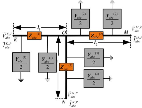
Figure 1. The three-terminal line model before the fault
