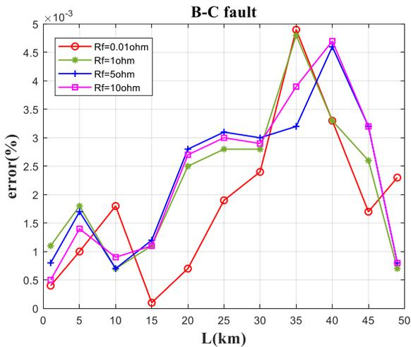
Figure 5. Results of the absolute fault location errors (in percentage), low impedance phase B to C faults with different fault locations and fault impedances
