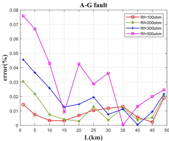
Figure 8. Results of the absolute fault location errors (in percentage), high impedance phase A to ground faults with different fault locations and fault impedances
