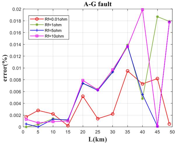
Figure 4. Results of the absolute fault location errors (in percentage), low impedance phase A to ground faults with different fault locations and fault impedances
