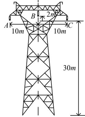
Figure 3. The tower structure of the untransposed transmission line
