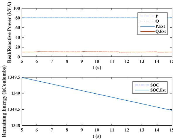
Figure 9: Actual and Estimated Power Output from Converter and SOC of Battery
