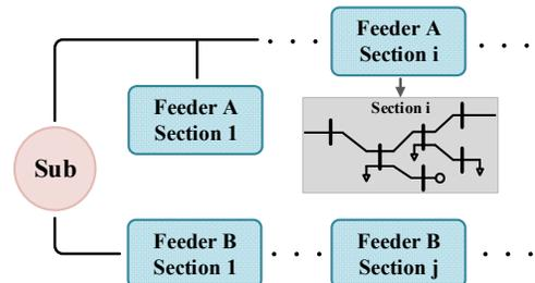
Figure 1: Partitioned Sections in Distribution System
