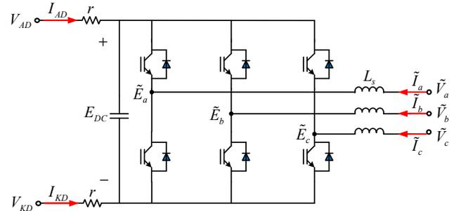
Figure 2: Circuit Diagram of DC-AC Converter
