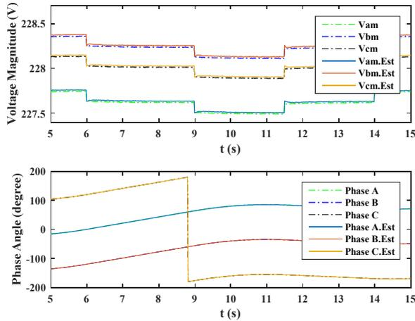
Figure 7: Actual and Estimated Voltage Phasor Measurements at B209
