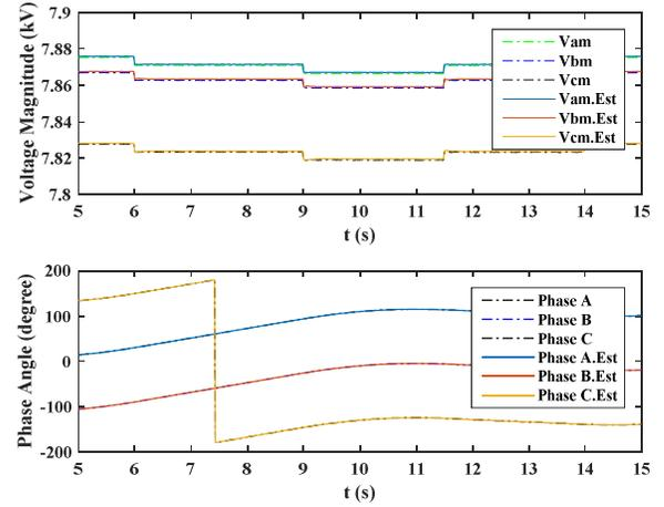
Figure 5: Actual and Estimated Voltage Phasor Measurements at B200
