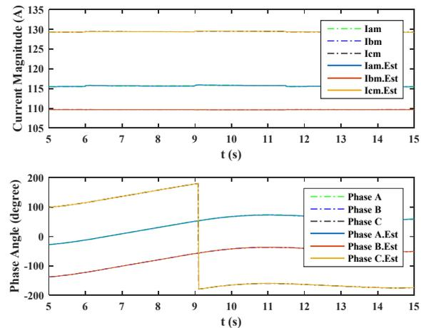
Figure 8: Actual and Estimated Current Phasor Measurements from B209 to B200
