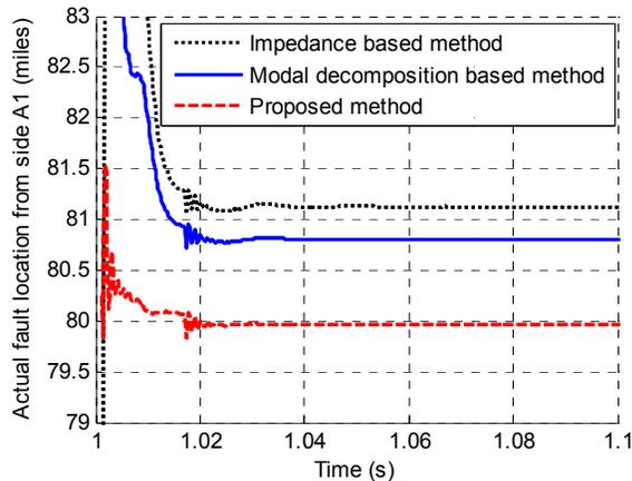
Figure 3. Fault locating results comparison, a 0.01 ohm phase A to neutral fault, 80 miles from side A1
