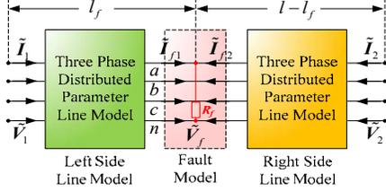
Figure 1. Phasor device model of two-terminal line with fault
