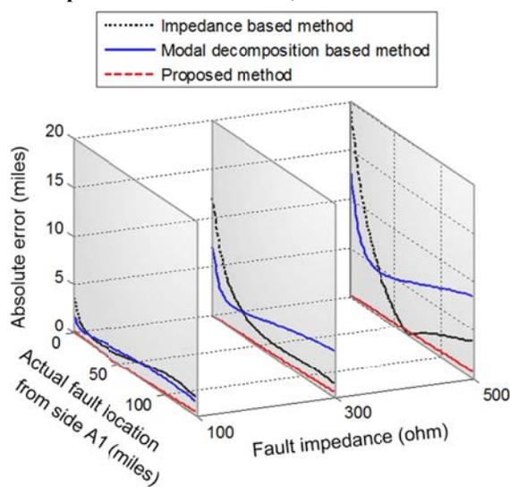
Figure 5. Fault locating results comparison, 100 ohm, 300 ohm and 500 ohm phase A to neutral faults, variable fault location
