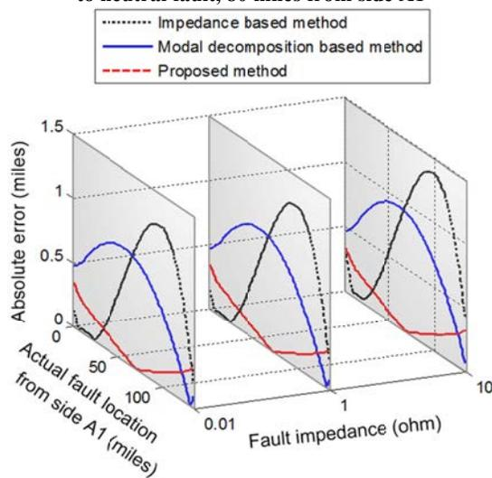
Figure 4. Fault locating results comparison, 0.01 ohm, 1 ohm and 10 ohm phase A to neutral faults, variable fault location
