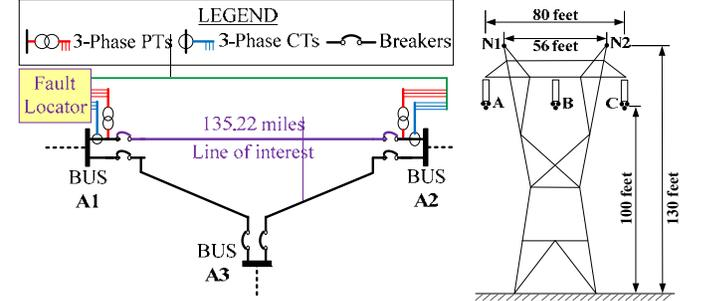
Figure 2. Example test system: two-terminal transmission line
