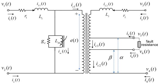
Figure 1. Model of transformer with inter-turn faults
