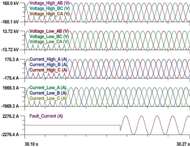
Figure 5. Transformer terminal measurements
