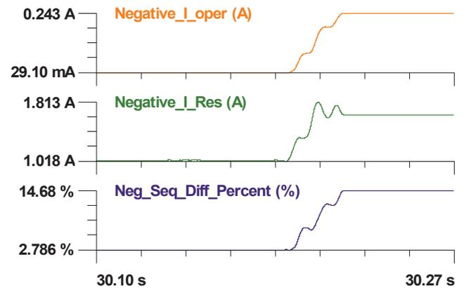
Figure 7. Results of negative-sequence differential method
