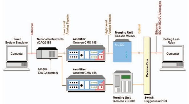
Figure 3. Hardware in the loop laboratory setup
