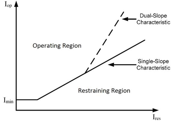
Figure 2. Percentage-differential protection method
