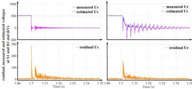
Figure 9. Voltage results: External fault event 3
