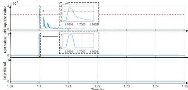
Figure 11. Protection results: External fault event 3
