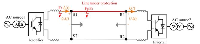
Figure 2. VSC-HVDC transmission system with faults
