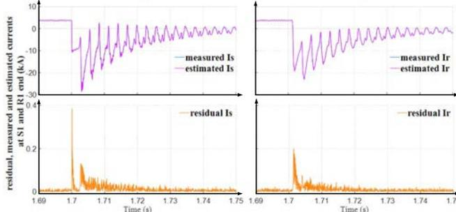
Figure 10. Current results: External fault event 3
