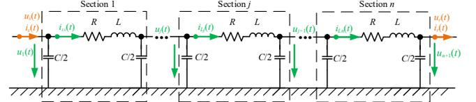
Figure 1. Transmission line model under protection
