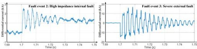
Figure 12. Differential current in the high impedance internal fault event and the severe external fault event
