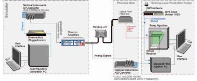
Figure 2. Laboratory hardware implementation
