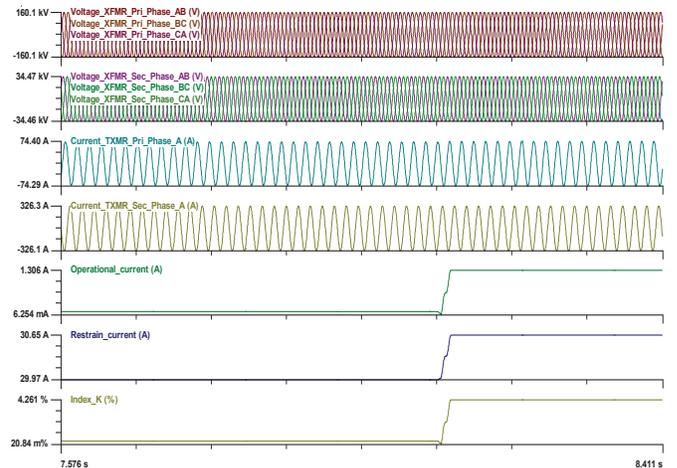
Figure 6. Differential protection for turn-ground fault near neutral terminal of transformer
