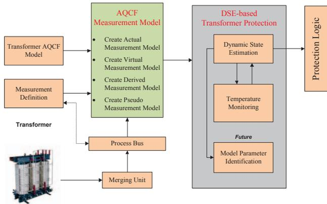
Figure 1. Overview of DSE-based transformer protection scheme
