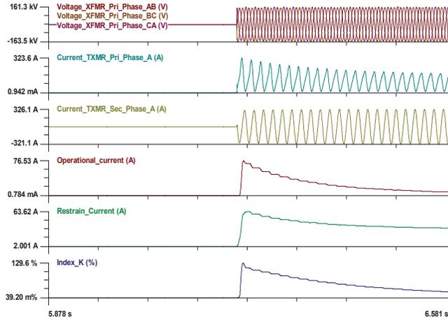
Figure 4. Differential protection scheme for inrush current
