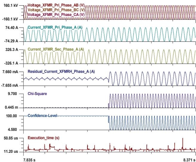
Figure 7. Proposed DSE-based protection for turn-ground fault near neutral terminal of transformer
