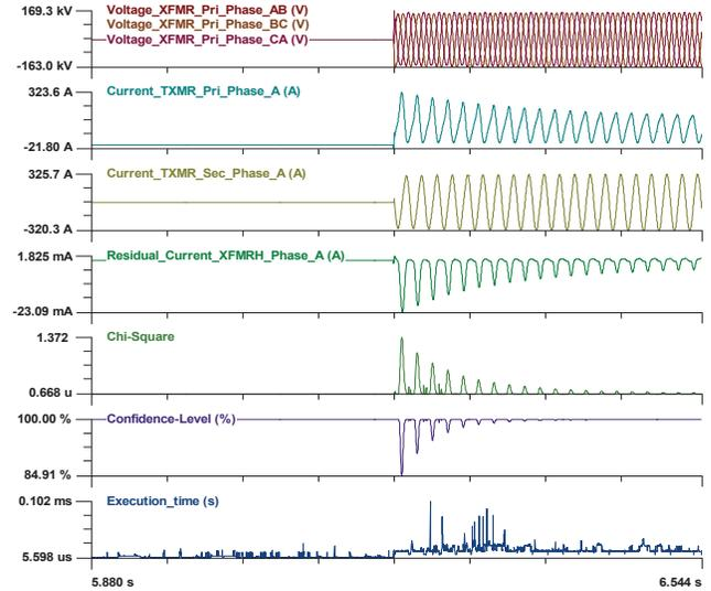
Figure 5. Proposed DSE-based protection scheme for inrush current of transformer
